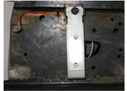
4. Slide the contactor back into position with battery + on the Contactor towards the batteries and reinstall the contactor nuts with the 11mm socket (**Figure 11-D**).
