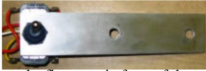
2. Install the contactor bracket onto the floor pan in front of the control. There are holes in the floor pan in which the bracket can be mounted with a 6MMx20 bolt, two 6MM washers (for top and bottom), a 6MM lock washer, and a 6MM nut (**Figure 9**).
