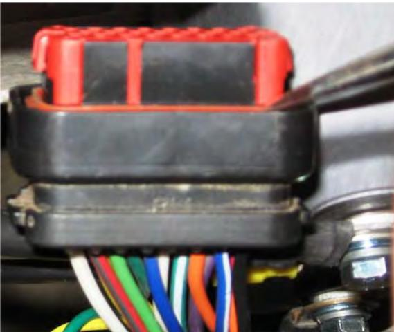
2. Connector should then look like the picture below (notice that the red tab insert is now extended above the black housing of the connector, but not completely dislodged from the connector).
