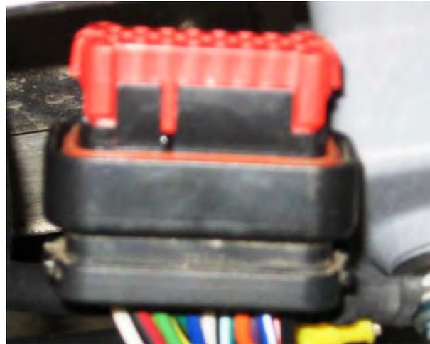
3. With red tab insert extended from housing (as shown above) pull the blue/white wire (pin 11) from the backside of the connector. Pin 11 is shown below.
