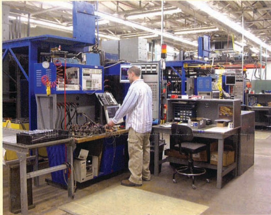
An FSIP technician performs a "true" load test to ensure the highest level of quality for every remanufactured control.
