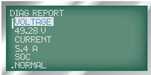
2. CALCULATED BATTERY CURRENT: displayed as 'CURRENT', the next line displays calculated current as 'HIGH', 'LOW' or the actual number in DC Amps.
