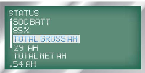
48. TOTAL NET AMP-HOURS: displayed as 'TOTAL NET AH', this is the total net Amp-Hours used for the life of the vehicle.
