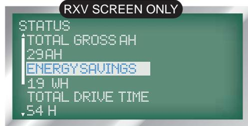
49. TOTAL RUNNING TIME: displayed as 'TOTAL DRIVE TIME', the next line displays the number of hours of running time (pedal down) on the vehicle in hours.
