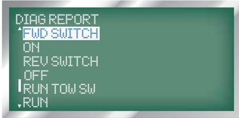
17. REVERSE SWITCH: displayed as 'REV SWITCH', the next line displays the switch position as 'ON' or 'OFF'.
