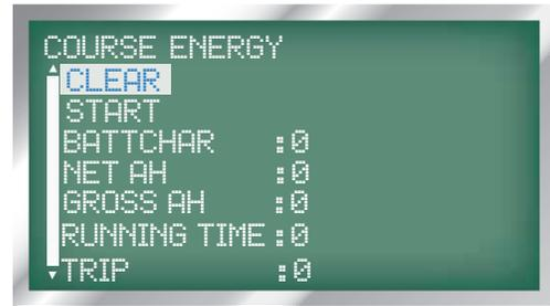
61. Scroll down to 'START' and press the enter key (button 3) to begin recording the energy consumption and begin driving.
