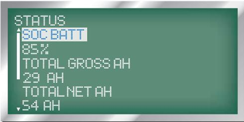
47. TOTAL GROSS AMP-HOURS: displayed as 'TOTAL GROSS AH', this is the total Amp-Hours used for the life of the vehicle.
