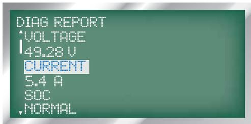
3. STATE OF CHARGE: displayed as 'SOC', the next line displays the state of charge for the battery pack as 'HIGH', 'NORMAL' or 'LOW BATT'.
