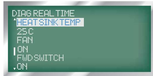
36. FAN function is displayed as "FAN", the next line displays whether or not the controller cooling fan is on or off.
