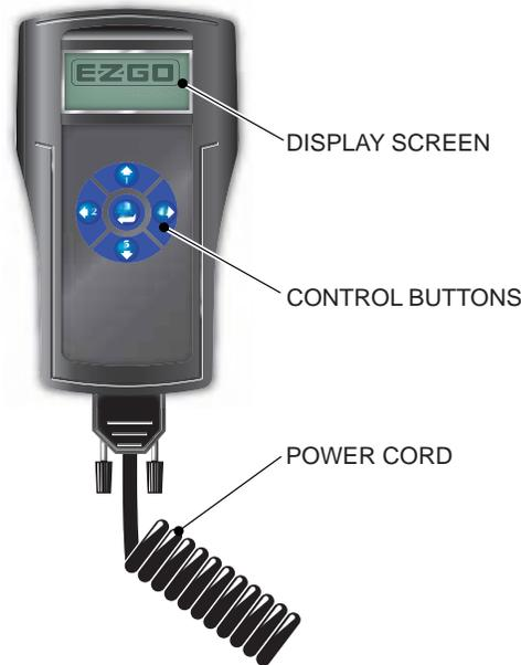
With the vehicle key switch in the 'OFF' position, the hand held diagnostic unit is connected to the vehicle by plugging the power cord connector into the receptacle (CAN) located under the vehicle cup holder. Turn the key switch on to power up the hand held. If the hand held shows 'no connection' or a blank screen, check the cord and the CAN connections and wiring.
