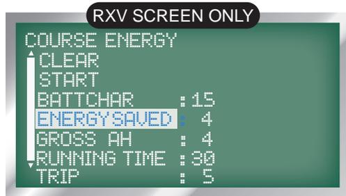
68. DISTANCE TRAVELED DURING RECORDING: displayed as 'TRIP', shows the distance traveled during recording in miles 'MI', whole number to the 10ths.
