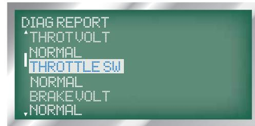
6. BRAKE SENSOR VOLTAGE: displayed as 'BRAKE VOLT', the next line displays the sensor voltage as 'LOW', 'NORMAL' or 'HIGH'.
