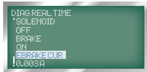
41. SOLENOID: displayed as 'SOLENOID', the next line displays the solenoid state as 'ON' or 'OFF'.
