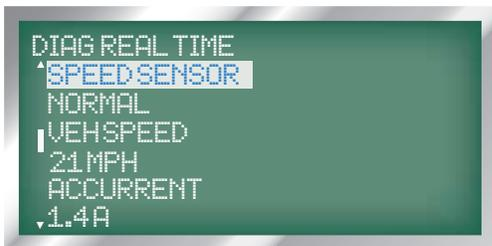
32. MOTOR VEHICLE SPEED displayed as 'VEHSPEED', shows the actual speed of the vehicle in miles per hour.
