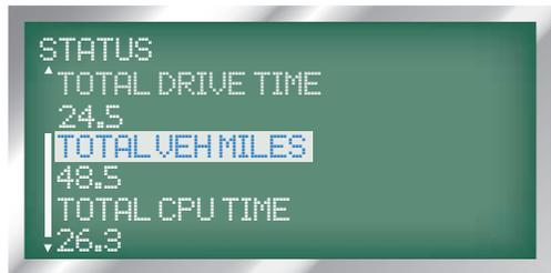
51. TOTAL LIFETIME OF THE CONTROLLER: displayed as 'TOTAL CPU TIME', the next line displays the total lifetime of the controller in hours and 10ths.
