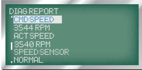
9. MOTOR ACTUAL SPEED: displayed as 'ACTSPEED', the next line displays the actual motor speed in RPMs.
