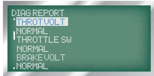
5. THROTTLE SWITCH POSITION: displayed as 'THROTTLESW', the next line displays the switch voltage as 'NORMAL' or 'ABNORMAL'.
