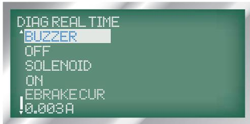
44. ELECTRIC BRAKE CURRENT: displayed as 'EBRAKECURR', the next line displays the brake current as a three place decimal in Amps; the brake current displayed below is 3 milliAmps.
