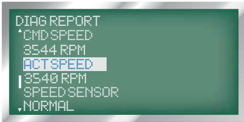
10. MOTOR SPEED SENSOR displayed as 'SPEED SENSOR', displays the status of the speed sensor. For troubleshooting see errors and warning chart.
