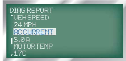
13. MOTOR TEMPERATURE: displayed as 'MOTOR-TEMP', the next line displays the internal motor temperature in °C.
