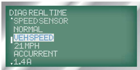
33. MOTOR CURRENT: displayed as 'AC CURRENT', the next line displays the AC current in Amps.
